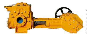
IP-145 IP-160 IP-175 Cylinder diameter : 145 mm 160 mm 175 mm Measured power : 7,5 kW 5,5 kW 7,5 kW Max capacity : 48 m3/h 60 m3/h 90 m3/h : 65 mwc. Max head 26 mwc. 22 mwc. -9.5 mtr. -9.5 mtr. Max vacuum : -9.5 mtr. Pump weight : 825 kg. 825 kg. 825 kg. 92% Efficiency : 92% 92%
