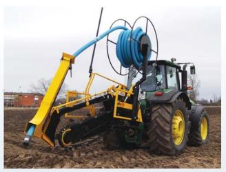
Trench widths are easily adaptable from 125mm to 400mm with digging booms for depths of up to 1.8m (71")
