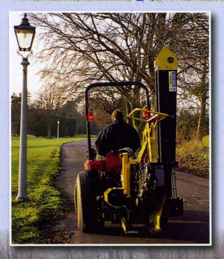
THE AFT45 FOR COMPACT TRACTORS is a strong lightweight trencher built to fit onto tractors of 15-34 Kw (20-45 hp).
